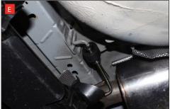
B) To remove the rest of the original GPF back system cut 80mm from the centre mounting bracket. De-bur this edge as the Scorpion adaptor will fit over it.
